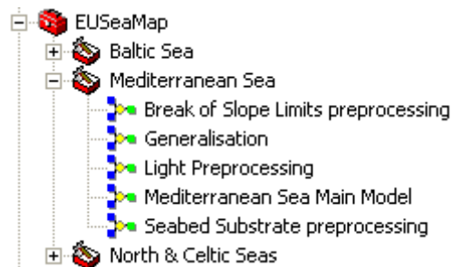
Figure 30 EUSeaMap Toolbox. It contains three toolsets (one per region), and each toolset contains at least one model, the main one. Here Mediterranean Sea toolset is opened. The main model is "Mediterranean Sea Main Model". The other models are not stand-alone, but are loaded by the main one.
