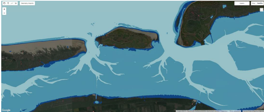
Figure 7 Coastline polygons for MHW, MSL, LAT estimated as 5%, 50%, and 95% percentiles of water occurrence images.
