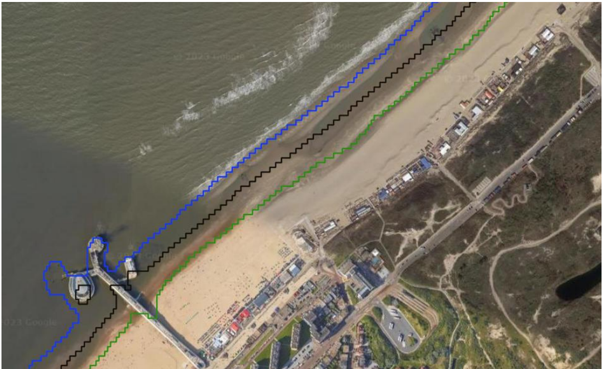
Figure 1 Example of coastlines at low-water, mean sea-level and high-water near Scheveningen in the Netherlands
