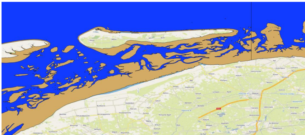
Figure 20 Inter-tidal area (Orange color), computed as set-difference of water at high-water and at low-water
