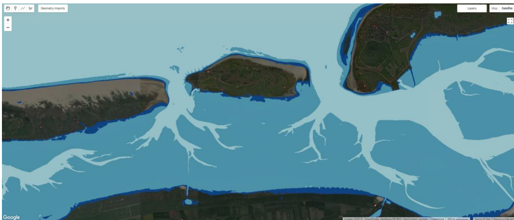
Figure 8 Coastline polygons for MHW, MSL, LAT estimated as 5%, 50%, and 95% percentiles of water occurrence images.
