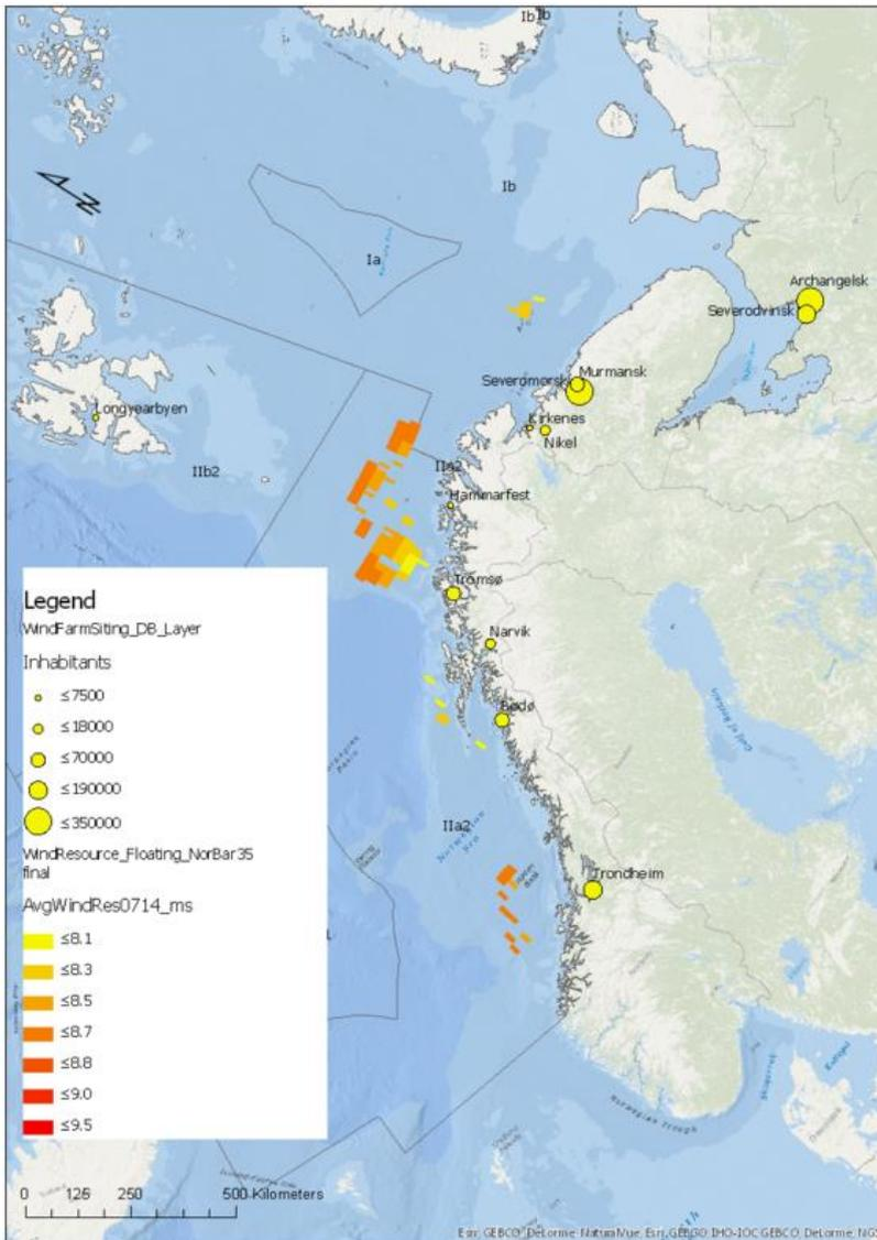
**Figure 9** Map showing the area with potential for developing (floating) offshore wind energy parks in the Norwegian Sea and Barents Sea, based on the first round of assessments within ‘SeaBasin Checkpoints – lot Arctic’. Also shown are human settlements that may play a role in this development.
