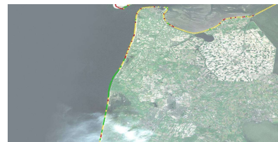
Accreting shoreline resulting from extensive sand nourishment (western Netherlands)
