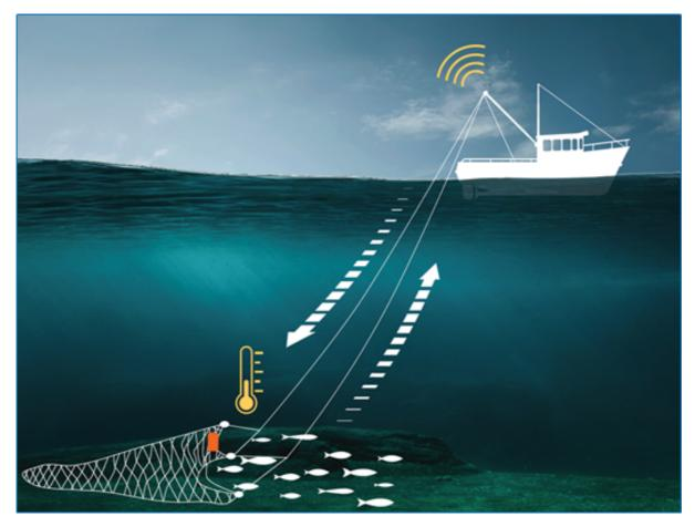
BDC supplies fishing vessels with sensors and deck equipment necessary to collect ocean data.
