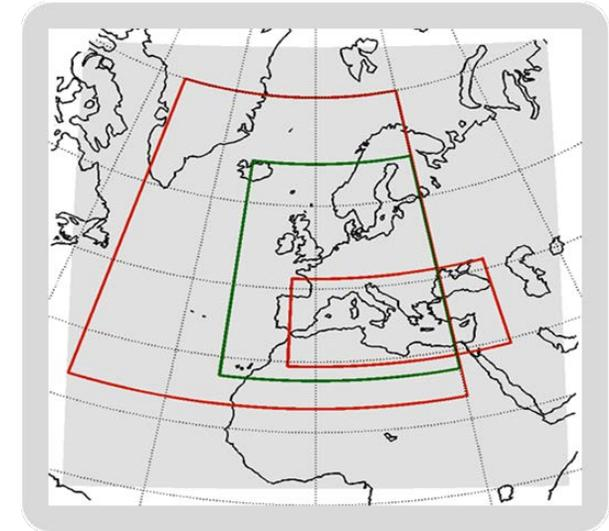
The set up and the domains of the wave model WAM
