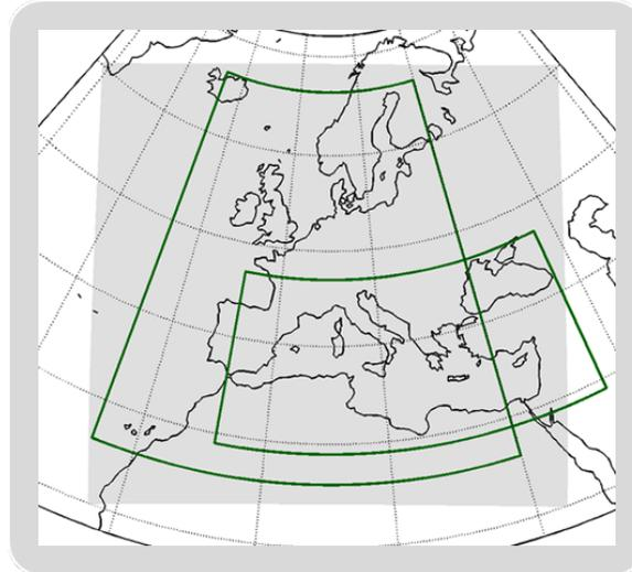
The set up and the domains of the atmospheric model Skiron
