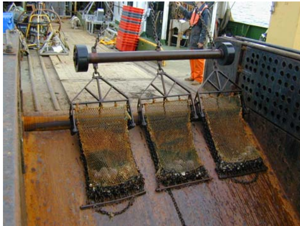
Figure 1. Trawls and dredges used for scientific sampling: (a) 2-metre wooden beam trawl; (b) rock dredge; and (c) scallop dredges.
