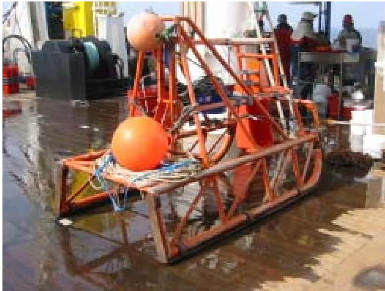
Figure 8. A ‘buff’ buoy attached to the rear of the sledge by rope.
