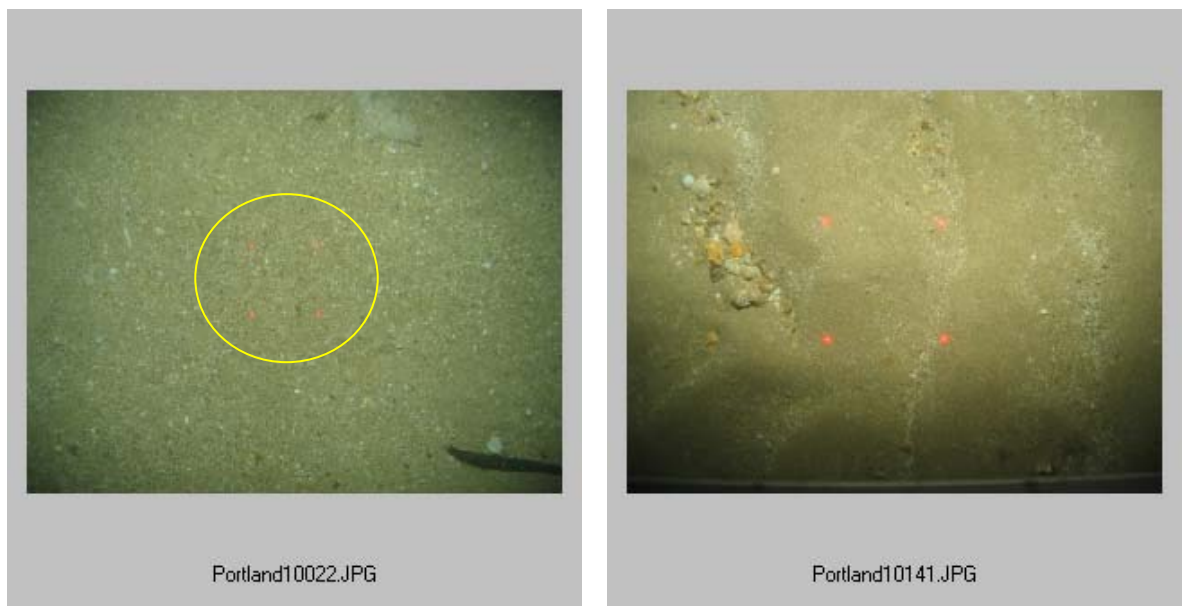
Figure 2. Spots from the same laser-scaling device used on a drop-camera frame. The camera is at a higher altitude above the seabed in the left image than in the right (photos by Cefas).
