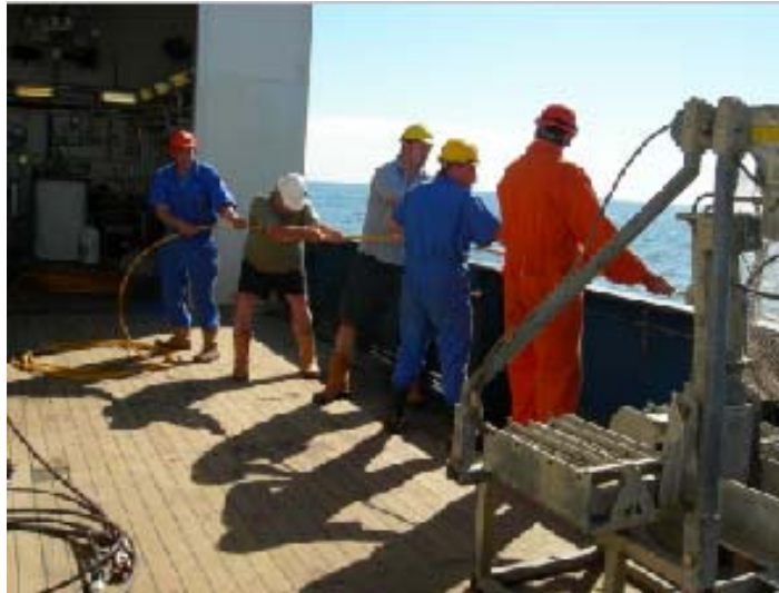
Figure 14. Deck crew recovering slack ROV umbilical. Note the last man in line is charged with coiling the umbilical neatly on deck as it is recovered.
