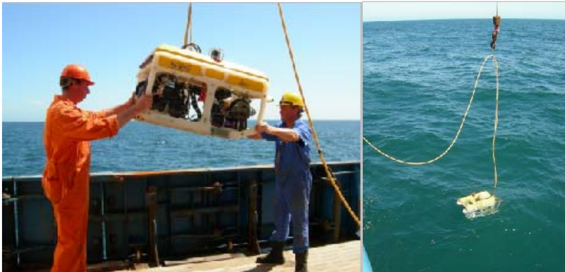
Figure 12. Manual handling of the ROV (left), and deployment by lifting strop and crane (right). At this point (right) it is safe to power-up the vehicle and test thrusters, prior to releasing the lifting strop. It is not safe to have the vehicle powered-up while it is being handled (left).
