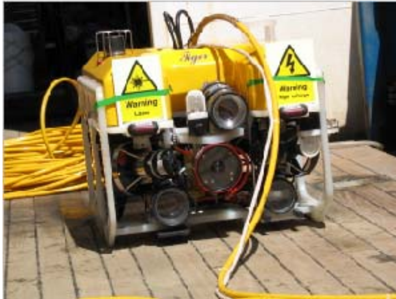
Figure 11. Warning notices displayed on ROV during live deck-testing.
