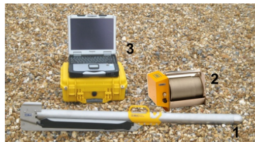
Figure 1 - Main components of a typical surface-towed sidescan sonar system.
