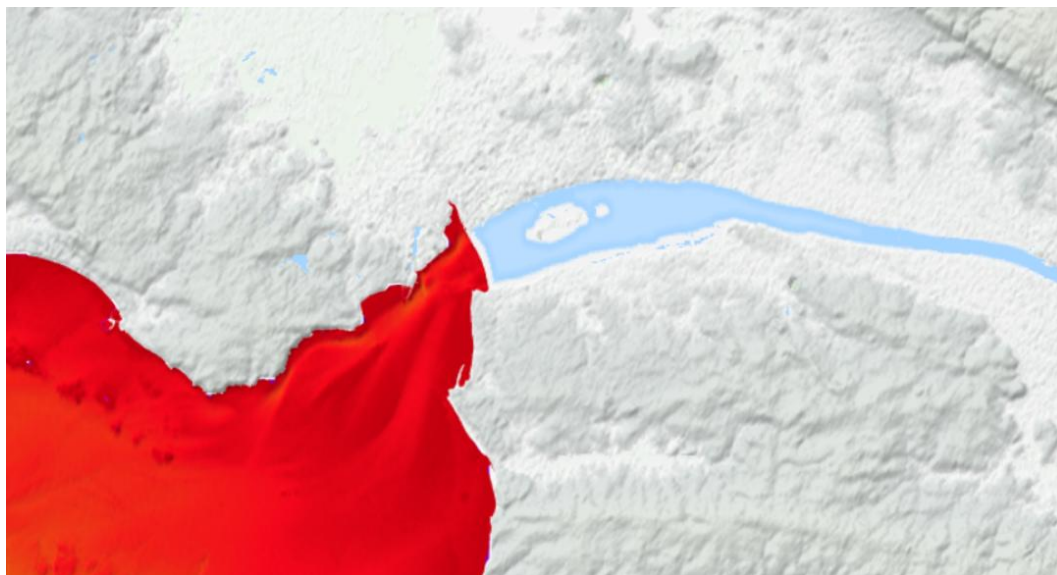
Figure 1 EMODnet gridded bathymetry (2023 release) for Loire River near saint Nazaire. Note the lack of bathymetry in the estuary.
