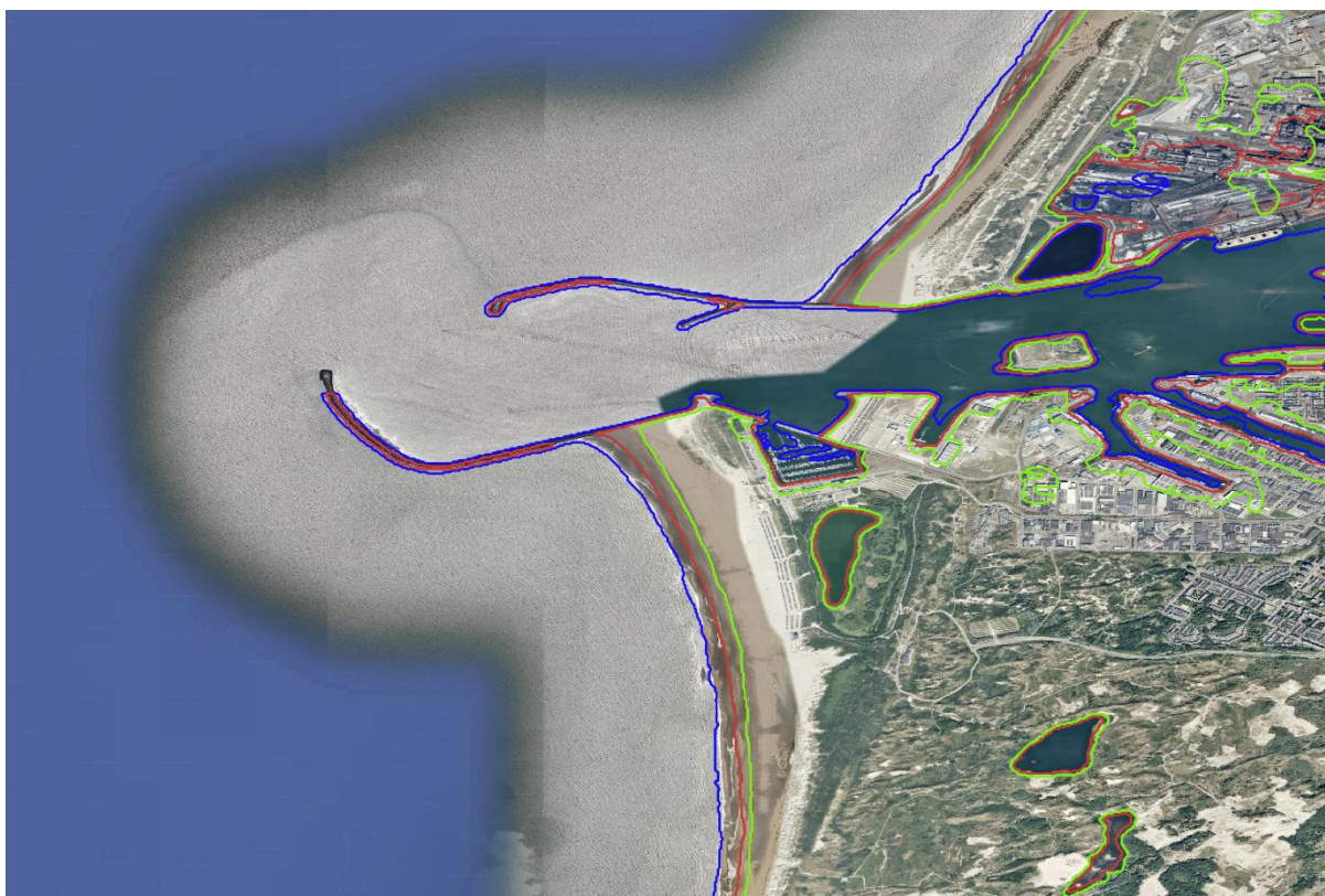
Figure 1 Example of coastlines at low-water, mean sea-level and high-water near IJmuiden in the Netherlands
